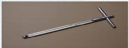
A soil tube or auger for soil sampling
